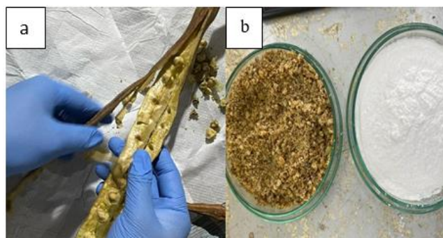
Figure 3. The researcher prepared malunggay for treatment (a. malunggay seeds, b. pulverized malunggay seeds and aluminum sulfate)
