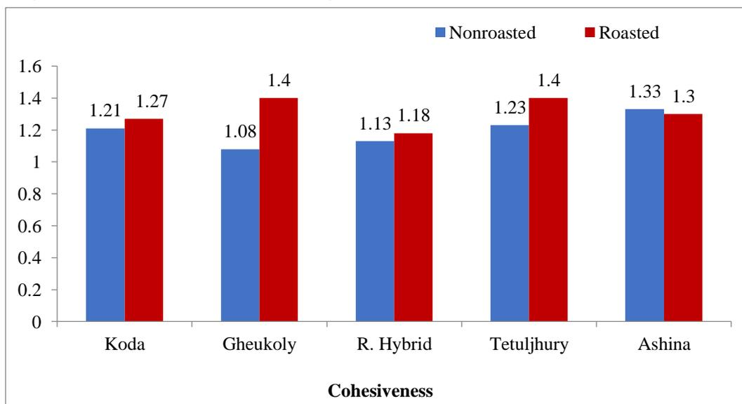
**Figure 4.** Cohesiveness for different samples expressed by Hausner-Ratio (roasted and nonroasted bean flour samples).
