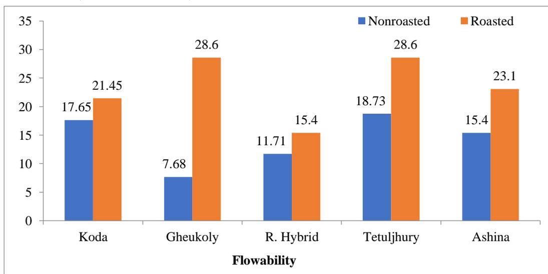
Figure 3. Flowability of different samples expressing by Carr-Index (nonroasted and roasted bean flour samples).
