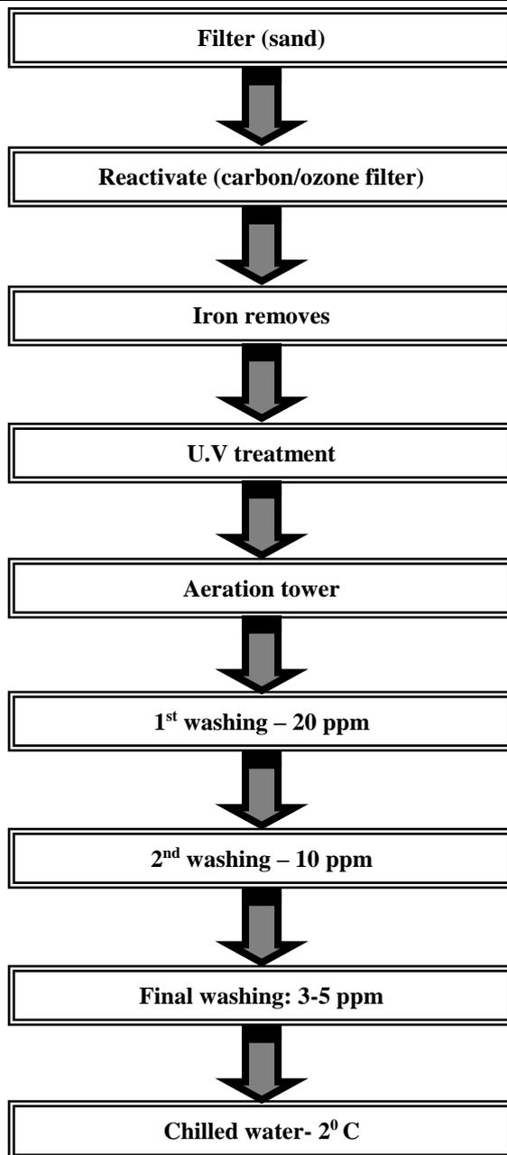
**Figure 3. Flow chart of water treatment system for washing shrimp.**
